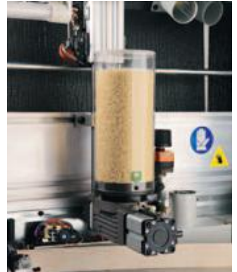
Pre-melting system QM-705 for EVA glue.
