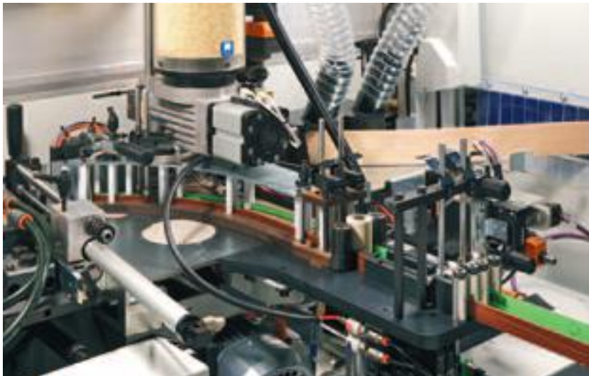
Automatic edge changement, managed by PC-Flat (opt).
