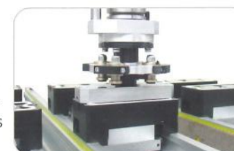
Automatic positioning of panel supports and vacuum cups by NC
