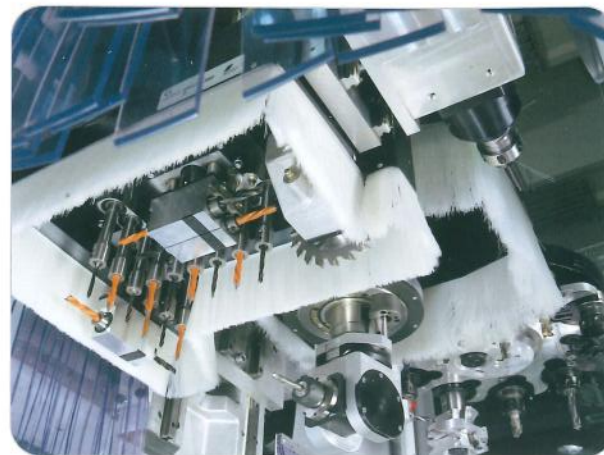
Testata a forare TFR18 con lama integrata TFR 18 boring head with integrated saw Cabezal de taladro TFR18 con sierra integrada
