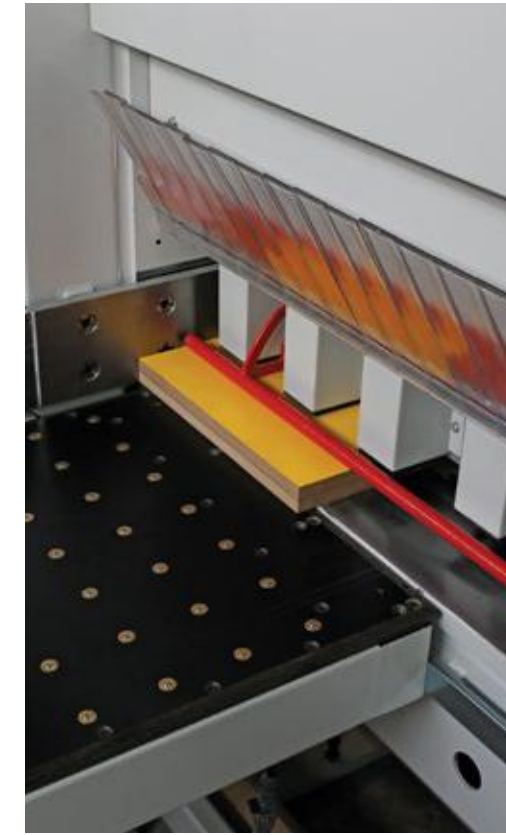
F Hava Yüzdürmeli Tablalar ve baskı, perde sistemi Transport tables with air blower and pressure, safety curtain system
