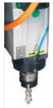
Fixed vertical motor dedicated to additional milling machining operations (slot, anti-splintering, etc.).
