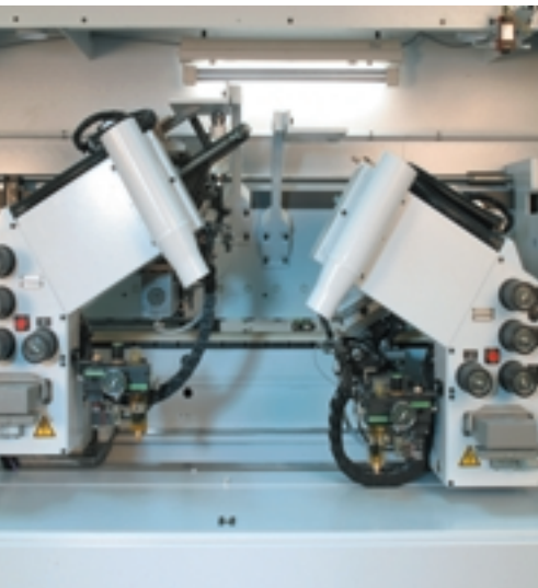
Profile trimming unit FK 11/FK 13 For processing edge overhang, as well as leading and trailing edges. Options: Chamfer / radius adjustment with stepless axis or manually.
