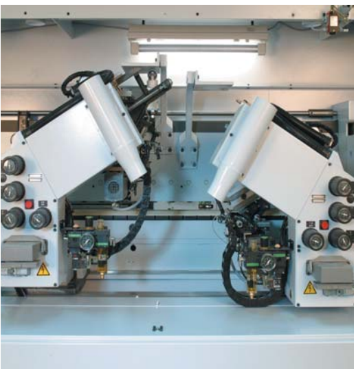
Profile trimming unit FK 11/FK 13 For processing edge overhang, as well as leading and trailing edges.*
