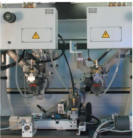
Profile trimming unit FF 12 For all-round finish trimming of workpieces, also those with postforming and softforming profiles.*
